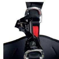
Using an additional carabiner (type HMS, e.g. SINGING ROCK BORA triple lock), the CAM CLEAN chest ascender can be attached to the harness.
