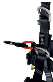
Specific EN 361 LADDER CONNECTION POINT on the front under the chest for connection to EN 353-1 fall arrest systems, which allows free movement on secured ladders and structures. If a fall is caught by the LADDER CONNECTION POINT, the auxiliary seams are ripped out and the point changes its position so that the user is not in danger of being turned head down.
